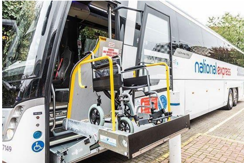
Figure 26 - National Express Coach with front Wheelchair Lift deployed
